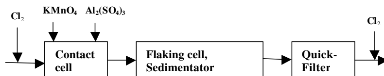
Figure 3. Daugava water treatment process [8].
